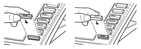
After programming the memory keys, label them with the supplied blank labels and key caps.<sup>†</sup>
