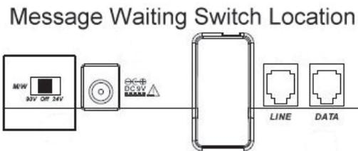
**Warning:** Setting this switch in a position other than OFF can cause this phone to function incorrectly. When enabled, this feature is for PBX systems, and not meant for direct Central Office (CO) interface. If connecting to CO telephone lines, make sure this switch is set to OFF.
